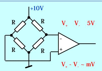
To measure 5mV signal with 1% error CMRR = 0.05/5000 = 100dB
