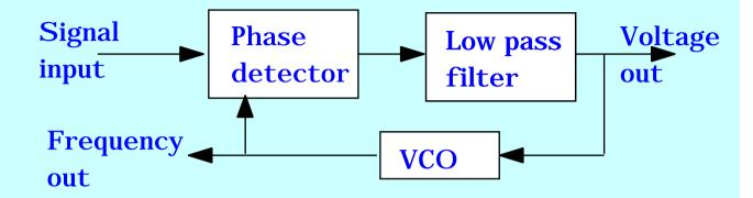
phase comparison with VCO generates error voltage...
