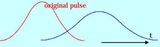
pulse after long distance in fibre
