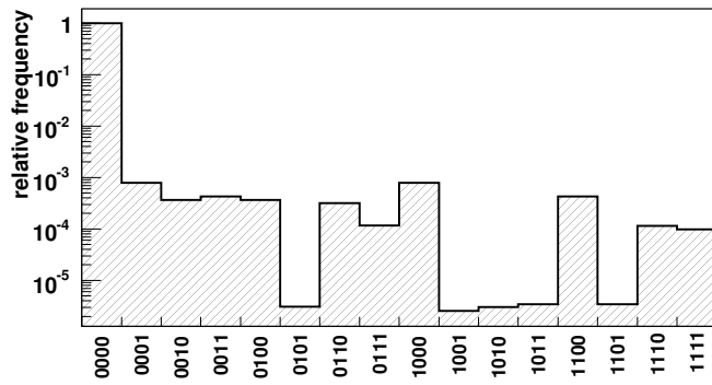
Figure 6: Pixels along each column are grouped into neighbouring fours. The digi patterns recorded are shown. For both figures minimum bias events are used with 400 events of pile-up.
