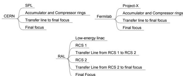
Figure 2: High-level breakdown of the three proton driver options for the IDS-NF.
