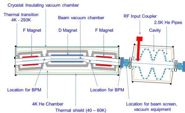
Figure 4: Schematic drawing of the FFAG cell.
