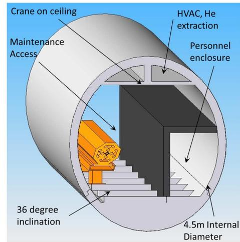
Figure 5: Cross-section of the decay ring tunnel showing the stepped floor and personnel enclosure.
