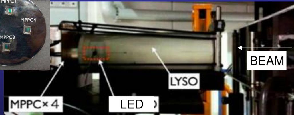
100 MeV electron beam tests at Tohoku University
