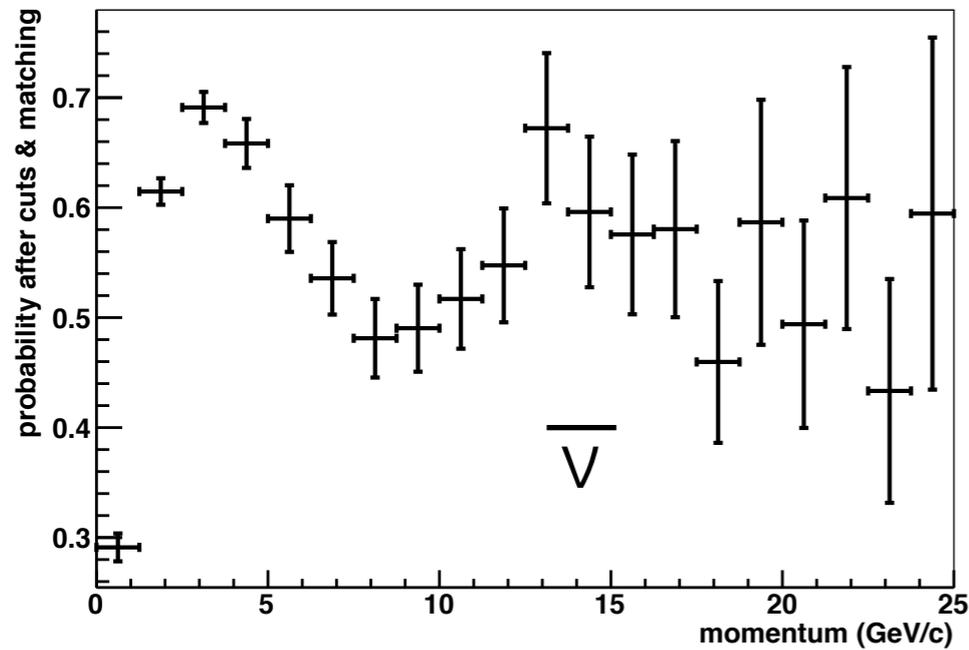
CC  $\nu_\mu$  muon reconstruction probability (after cuts)
