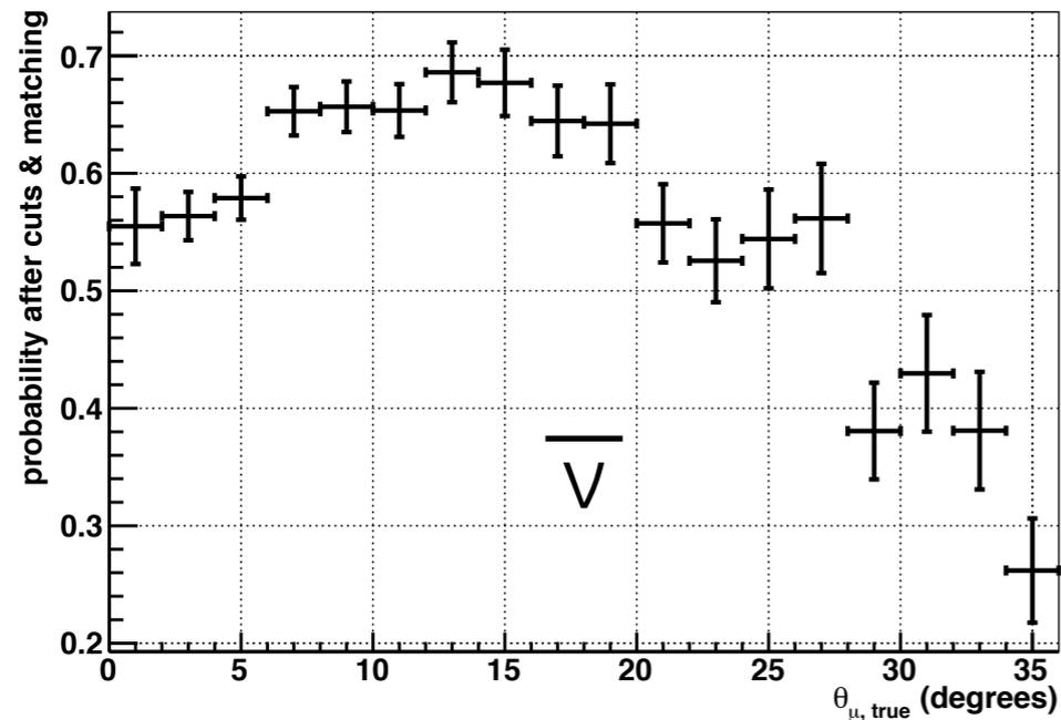
CC  $\nu_\mu$  muon reconstruction probability (after cuts)
