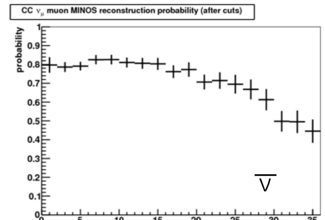
At low momentum or large angles the charged particle does not make it to MINOS ND
