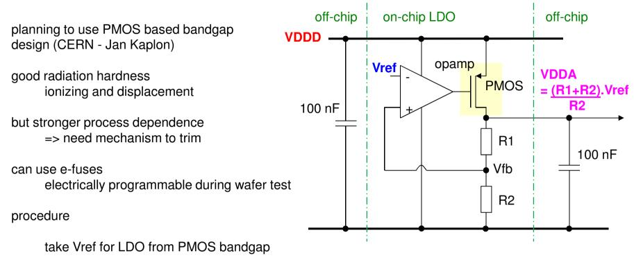
use I2C register to trim VDDA to desired value during wafer test
