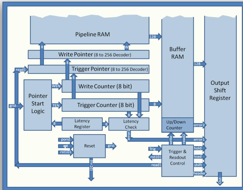
**Figure 11.** Pipeline Control Logic
