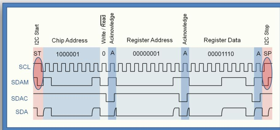
Figure 14. I2C Write Transaction
