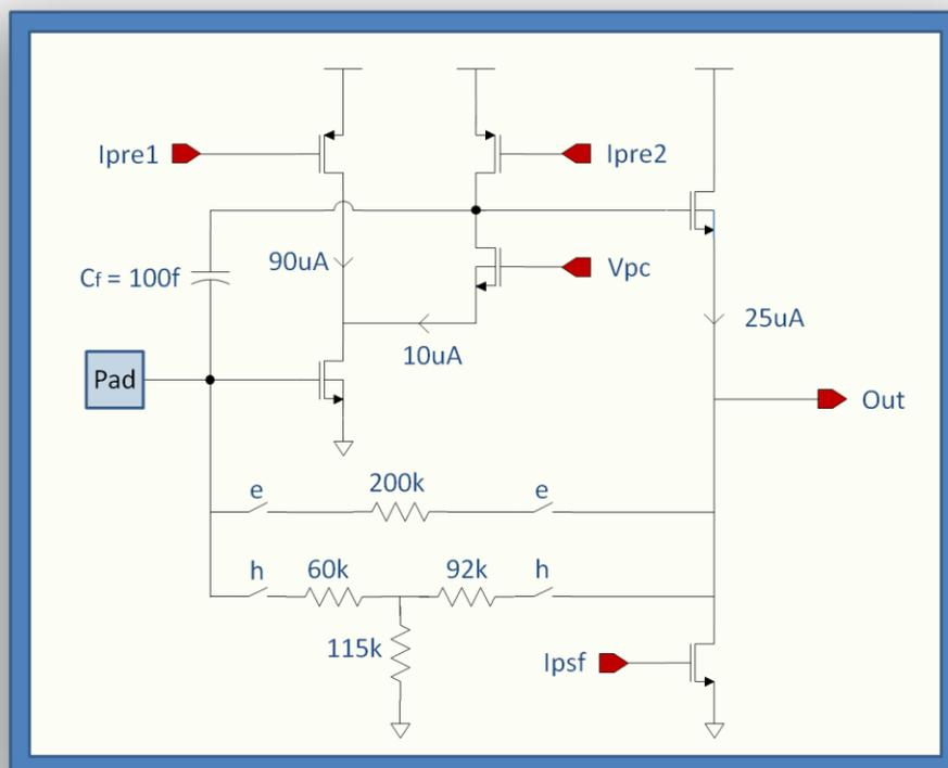
Figure 3. Preamplifier Schematic
