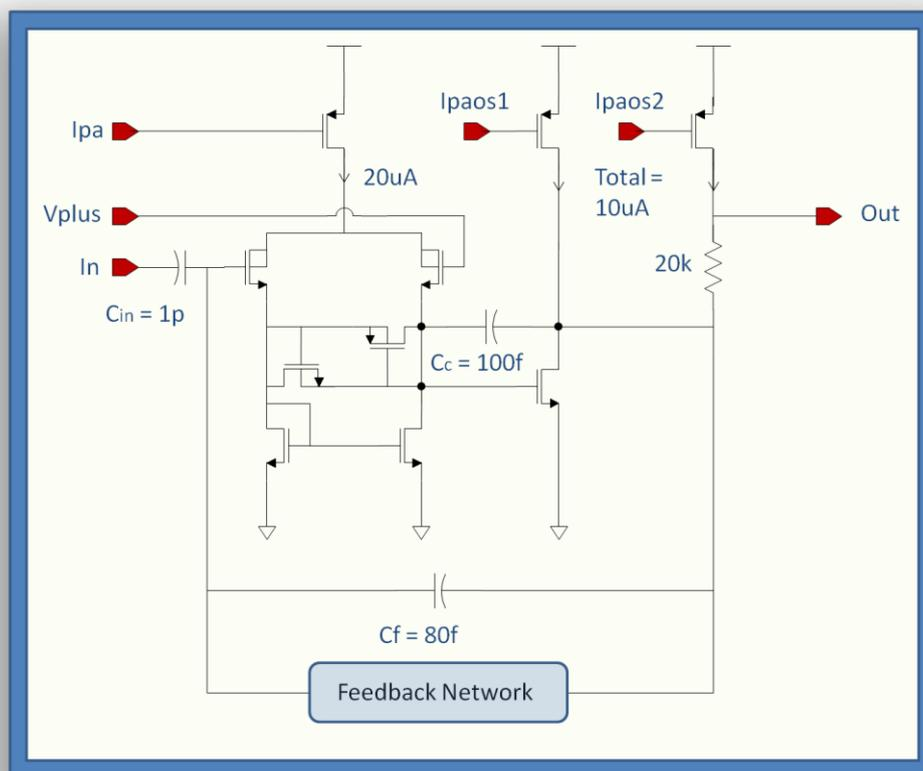
Figure 4. Postamplifier Schematic
