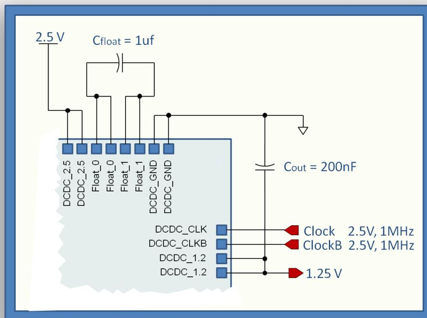
**Figure 18.** Connections for DC-DC Converter.
