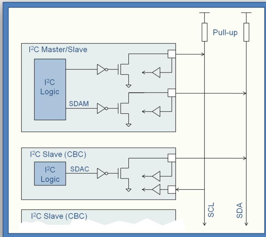
**Figure 13.** I2C Master/Slave Configuration
