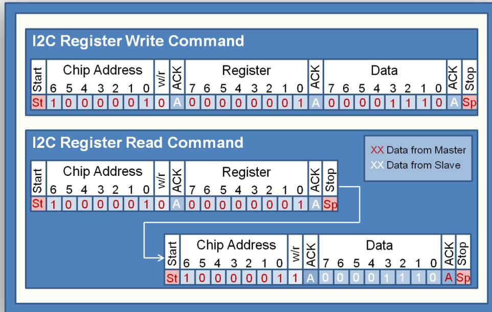
Figure 15. I2C Write/Read Transaction
