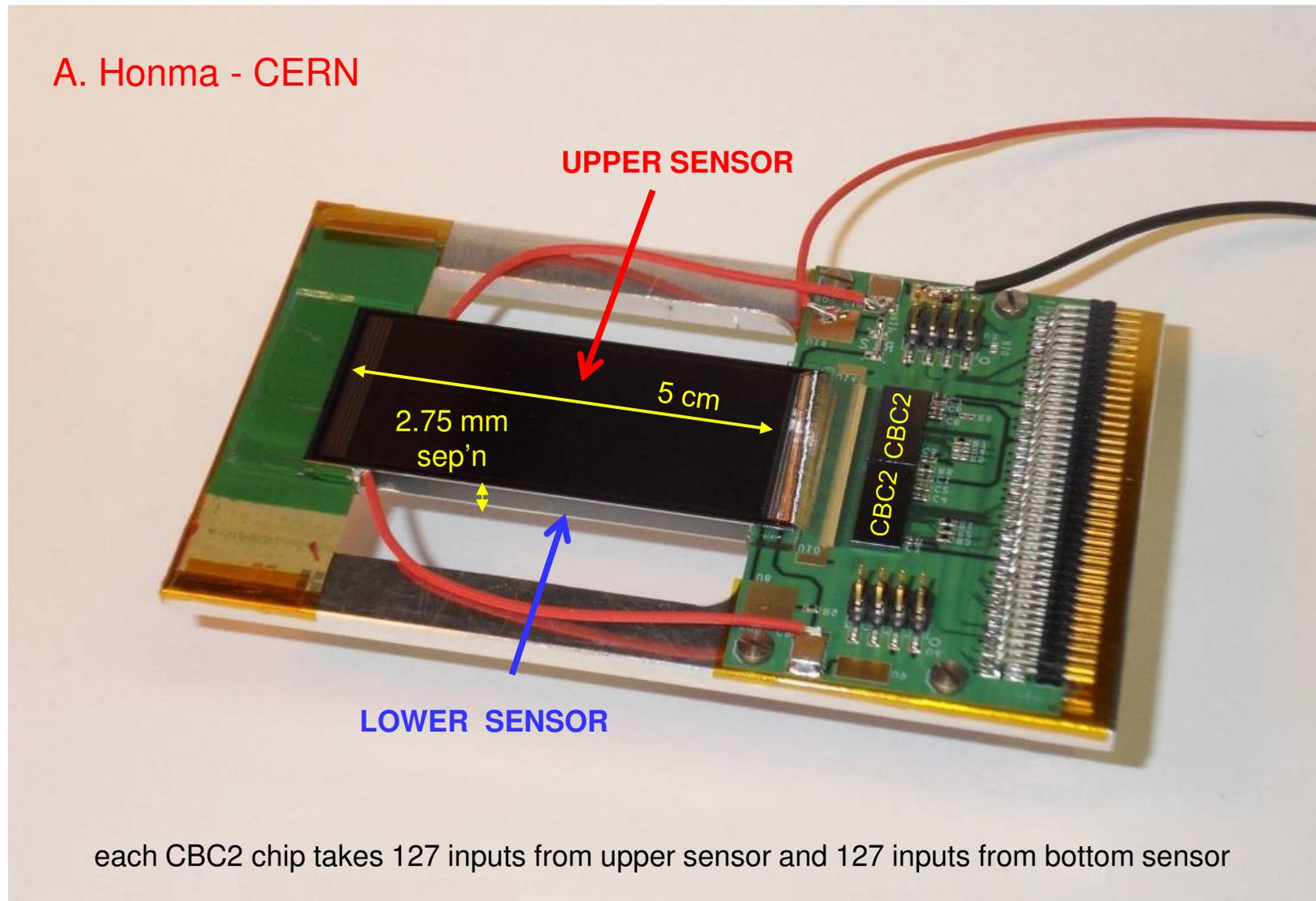
each CBC2 chip takes 127 inputs from upper sensor and 127 inputs from bottom sensor
