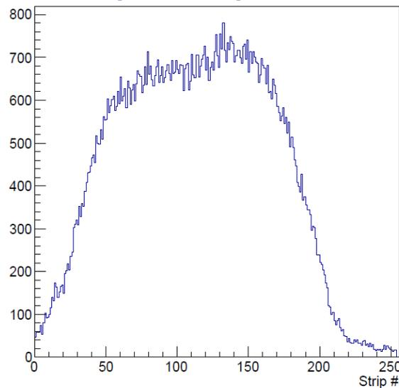
angular scan of CNM module in beam
