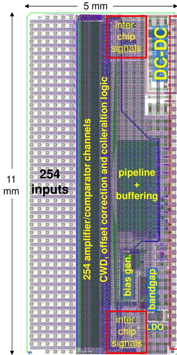
C4 bump-bond layout, 250  $\mu\text{m}$  pitch, 19 columns x 43 rows
