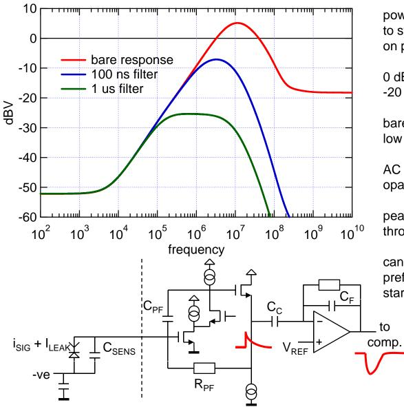
power supply rejection at postamp output to swept frequency sinusoidal waveform on positive supply rail
