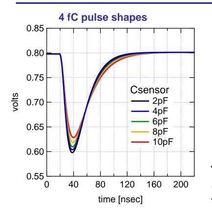
trade-off between power and noise thin sensors, long strips will need more power to get less noise pulse shape tuned to keep risetime ~ constant as  $C_{\mbox{\scriptsize SENSOR}}$  varies by increasing current in input FET
