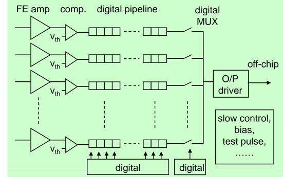
simpler synchronous system no FE timestamping data volume known, occupancy independent (no trigger-to-trigger variation)
