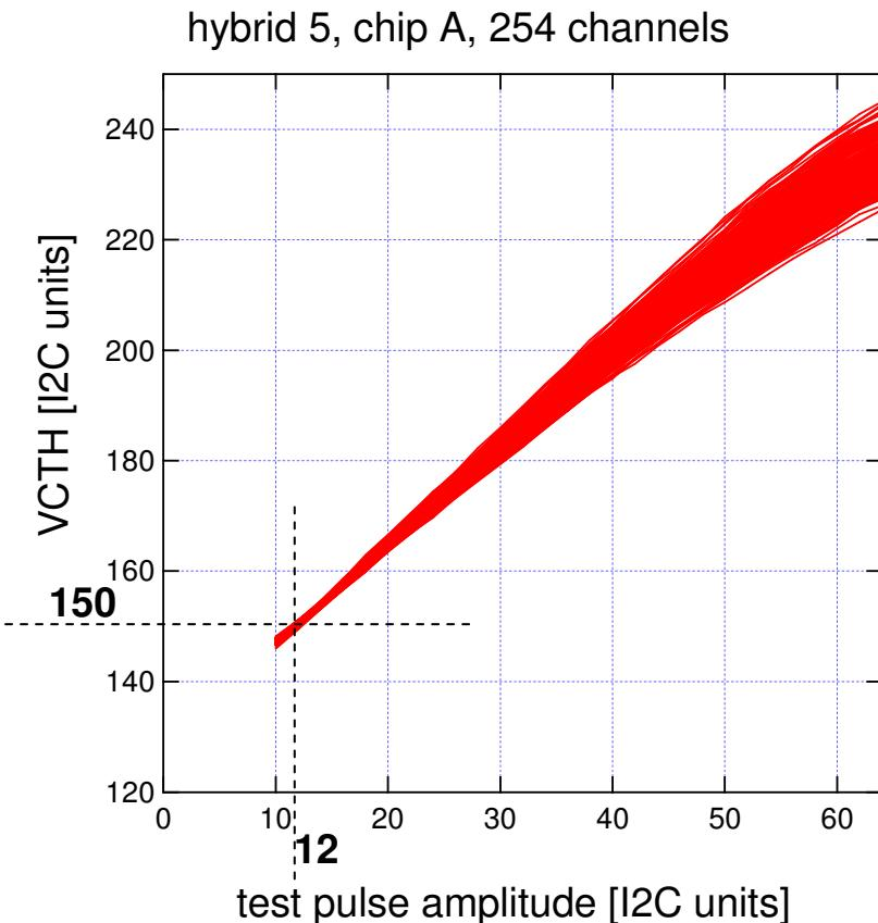
sweep test pulse amplitude and measure s-curve mid-points by sweeping global comparator threshold voltage VCTH
