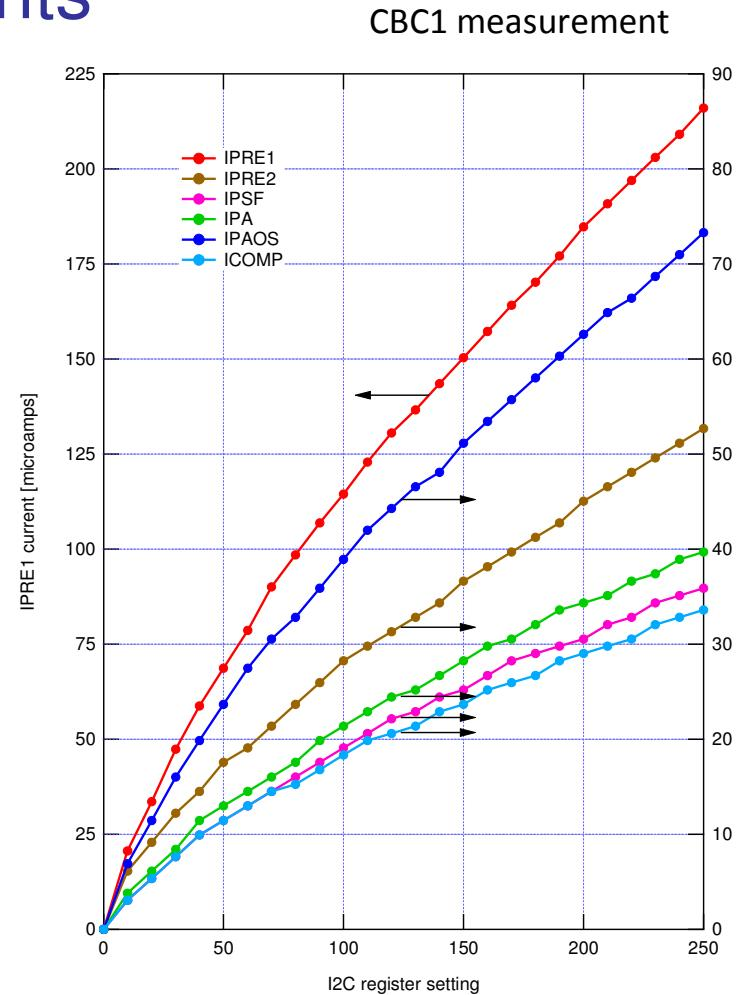
total current (all channels) measured in supply rail
