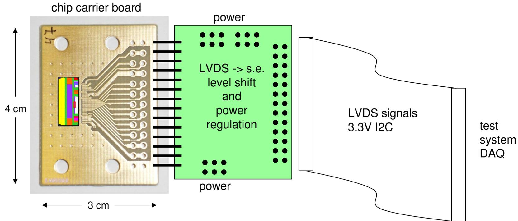
use probe pads to wire-bond chip to simple carrier board
