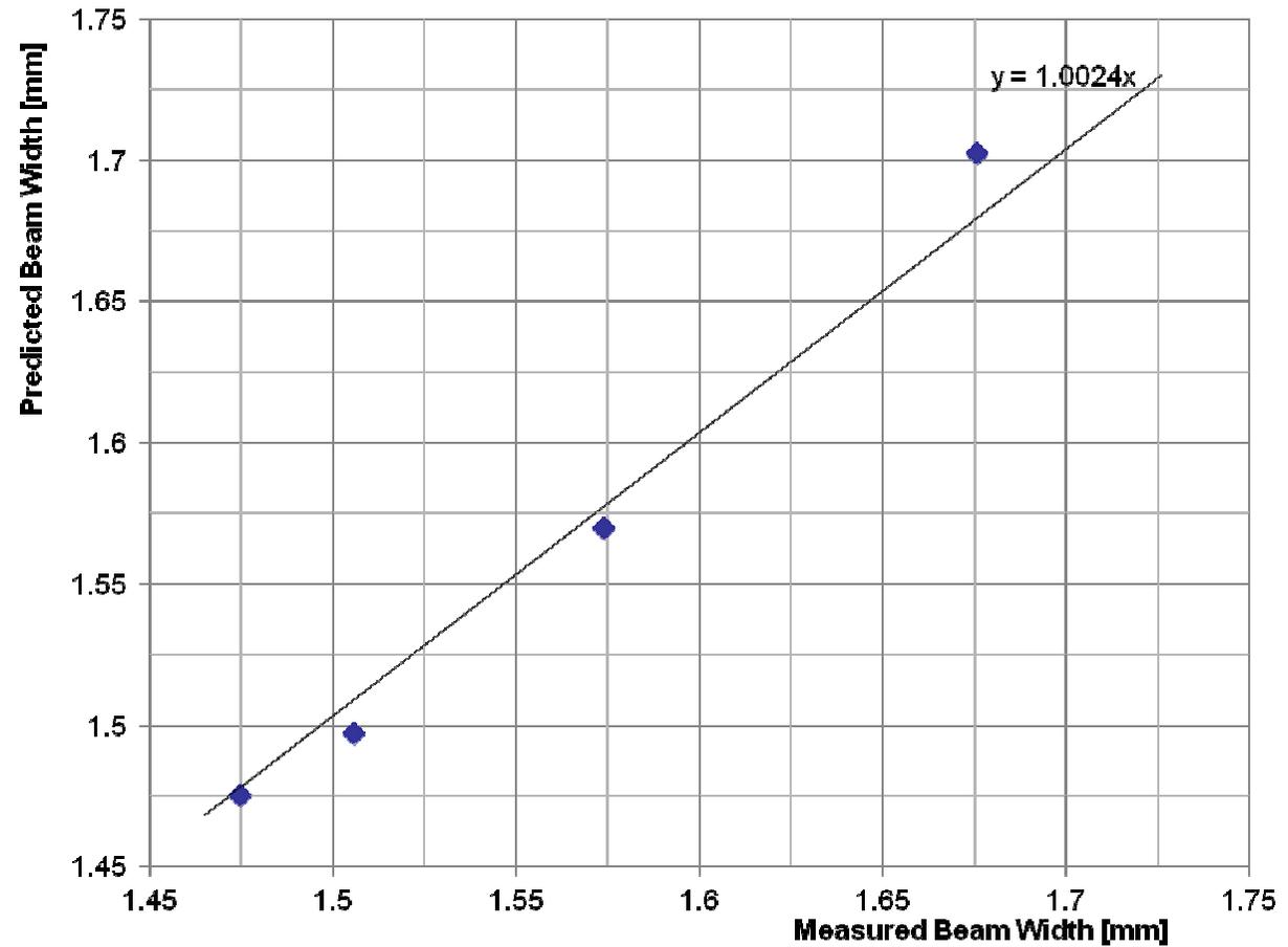
predicted beam width = normal incidence beam width /  $\cos \theta$
