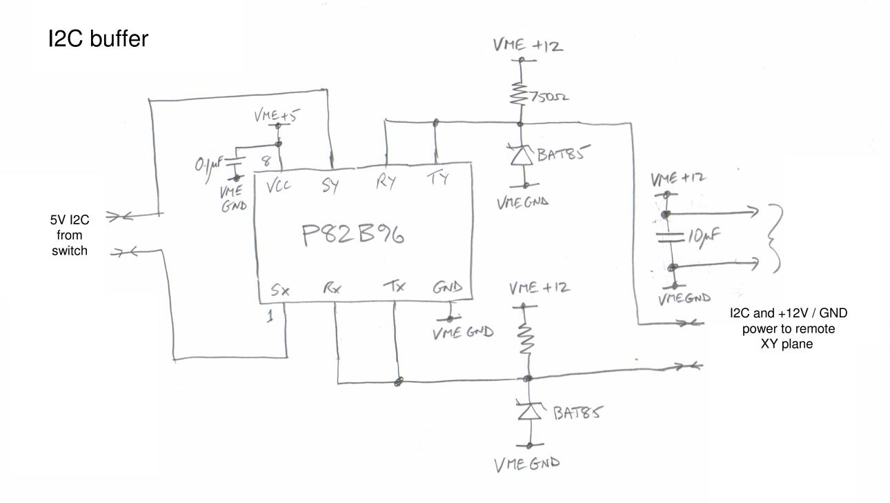
The 12V power from the I2C hub is transmitted along with the I2C signals, to power the P82B96 and the opto-isolate stage in the XY plane
