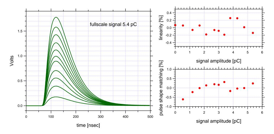
pulse shape matching in spec., linearity outside by factor ~2
