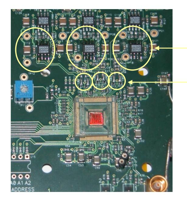
mismatch of stray O/P capacitance likely due to signal routing on test card
