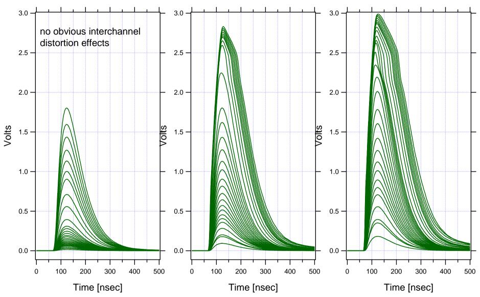
Differential pulse shapes – all 3 gain channels compared – gain ratios 1:5.6:11.3 (cf 1:6:12)
