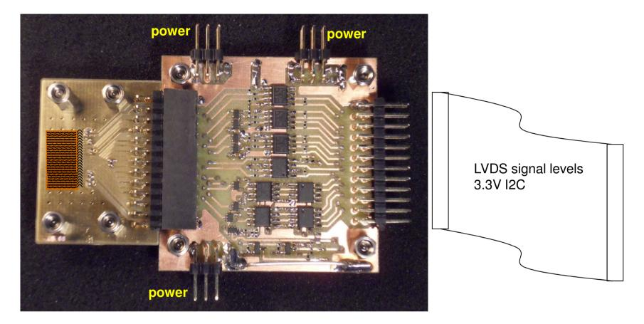
use wafer probe pads to wirebond single CBC2 die to carrier (CBC2 chips from diced wire-bond (XFEL) wafer) interface board tested and working
