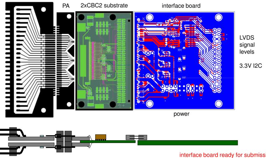
2xCBC substrate + PA (both sides) becomes device under test pluggable charge inject board allows different external capacitance
