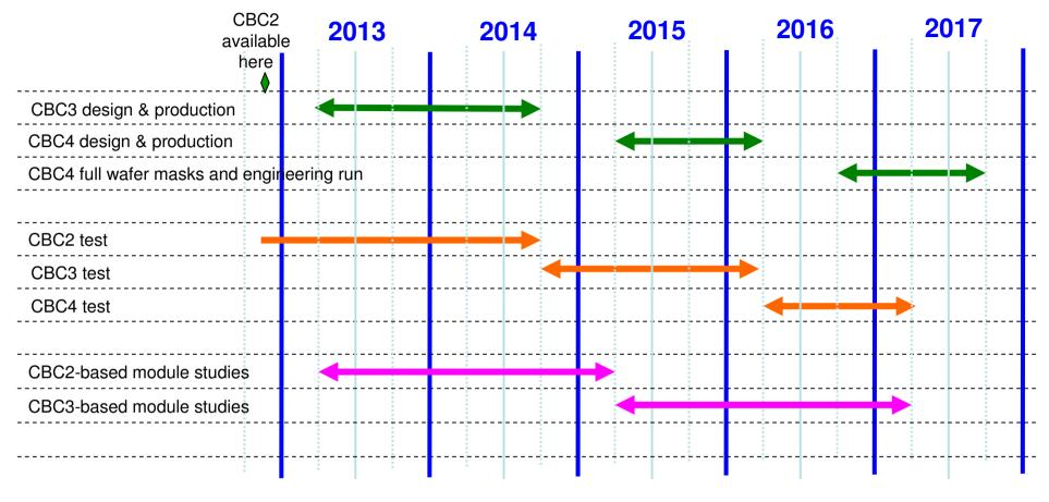
CBC3 should be very close to final chip – available late 2014 incorporate architecture to transmit stub addresses slow ADC for on-chip monitoring
