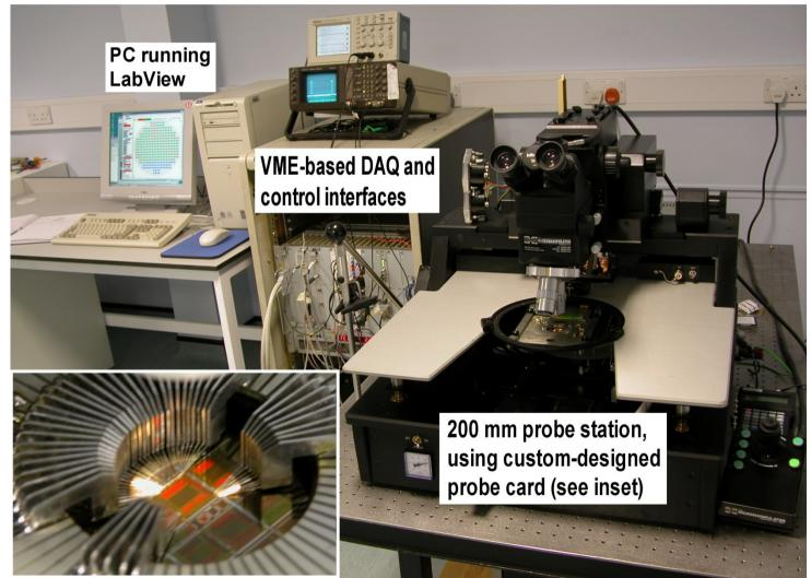
Micromanipulator 8 inch semi–automatic probe station
