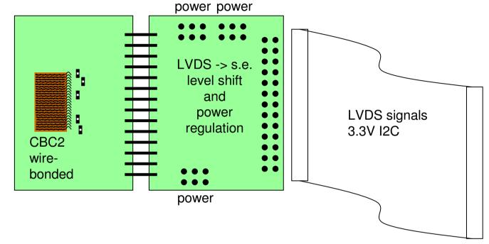
use wafer probe pads to wirebond single CBC2 die to carrier (CBC2 chips from diced wire-bond (XFEL) wafer)
