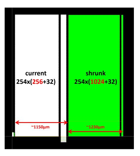
It is possible to have 4 times the memory in the existing area without widening the chip.
