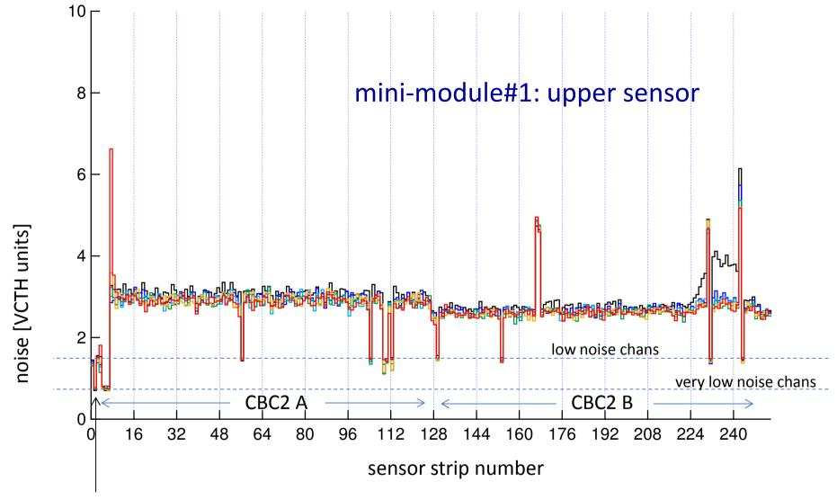
this one corresponds to the broken wire - what about the others? to diagnose look at test pulse response behaviour
