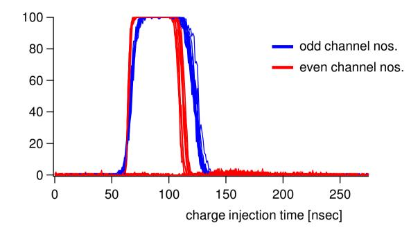
slower edge times for odd channels (lower sensor) => slower pulse shape => higher capacitance
