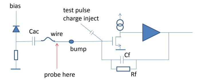
behaviour observed consistent with failure of connection between strip and amplifier poor wire contact? something wrong with sensor? failed bump-bond seems the most likely?
