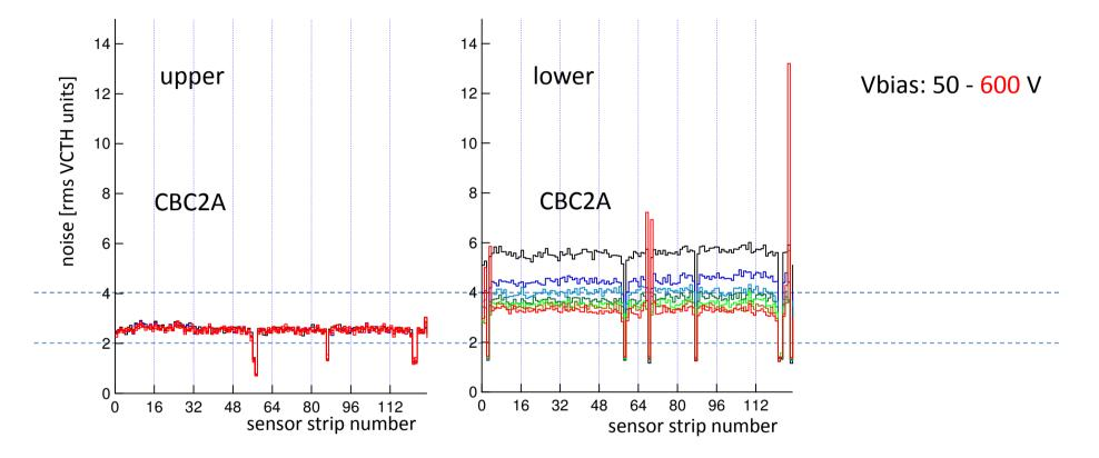
similar behaviour, but lower sensor doesn't get to as low levels as upper before noisy strips start to develop
