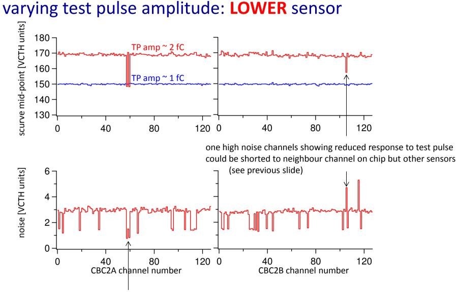
pair of very low noise channels on this sensor also showing no response to test pulse
