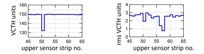
for a normally behaving channel (strip 50), grounding the wire-bond pad which is connected (via bump-bond) to CBC input, means that that channel no longer responds to the test-pulse
