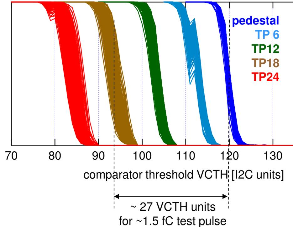
raw s-curve data shows effects of comparator threshold non-linearities
