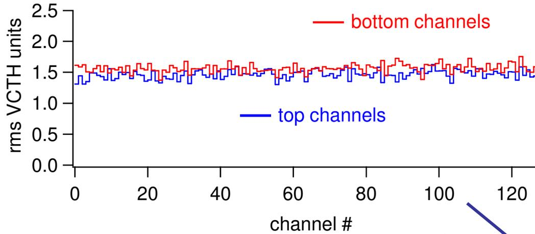
slightly higher noise observed for channels on bottom surface of hybrid
