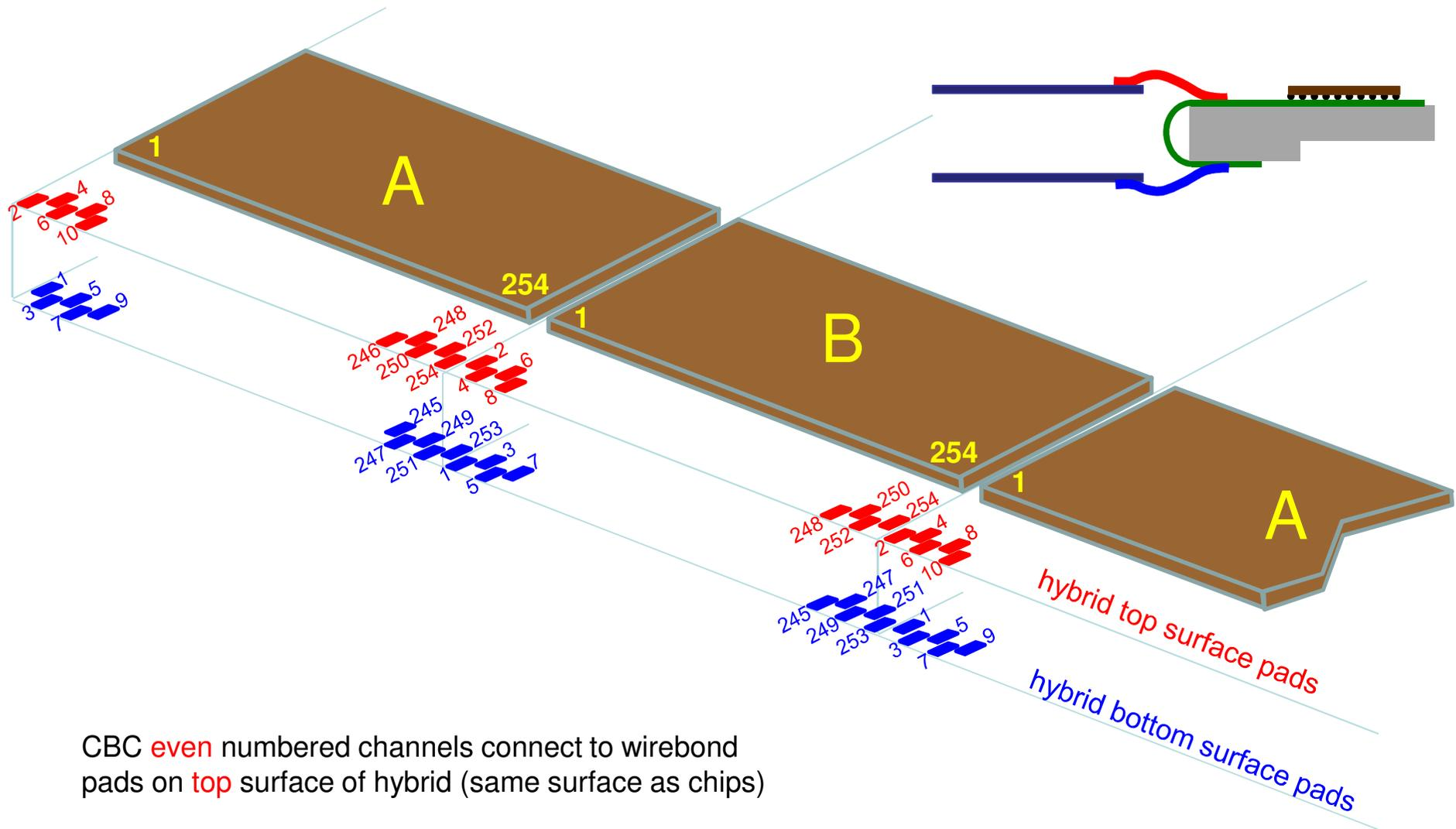
CBC **even** numbered channels connect to wirebond pads on **top** surface of hybrid (same surface as chips)
