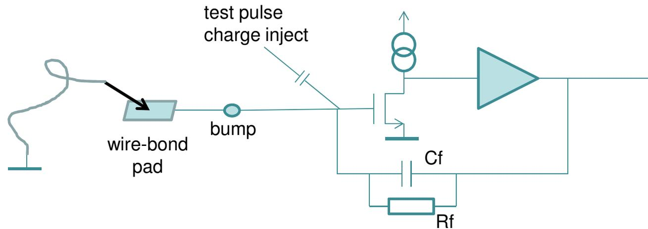
goal is to verify all channels connected via bump to wire-bond pad array
