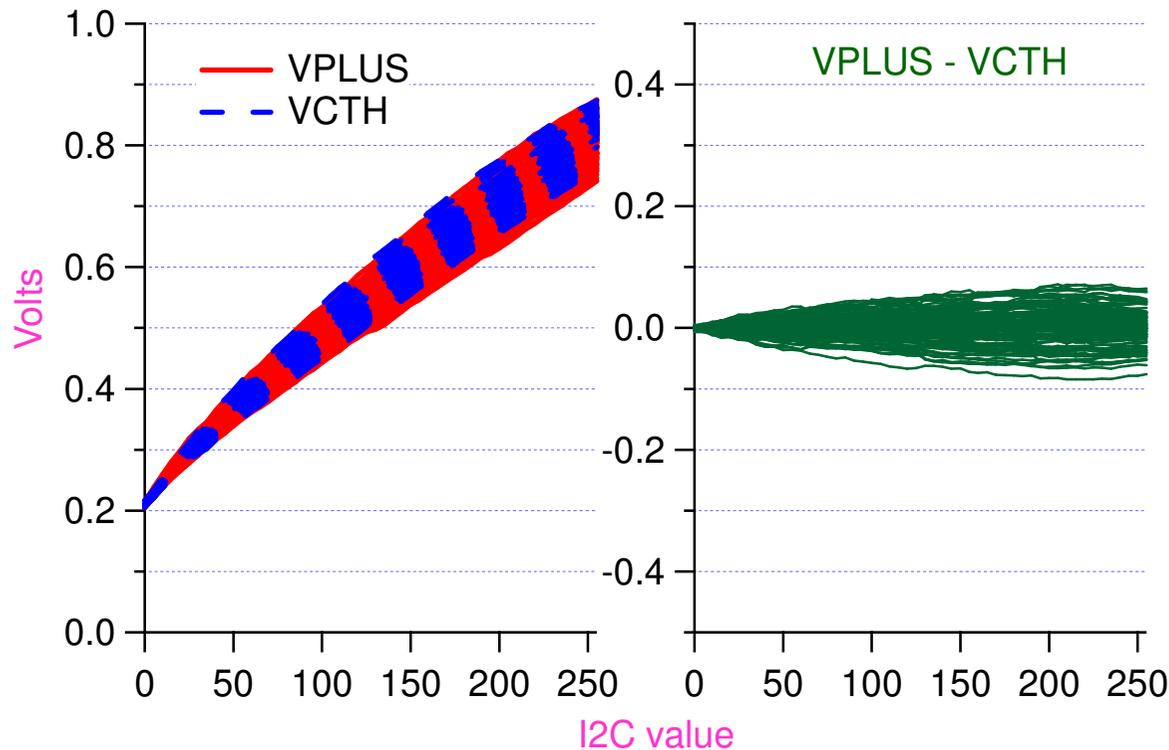
wafer test measurements show large spread in VCTH and VPLUS vs I2C setting, chip-to-chip
