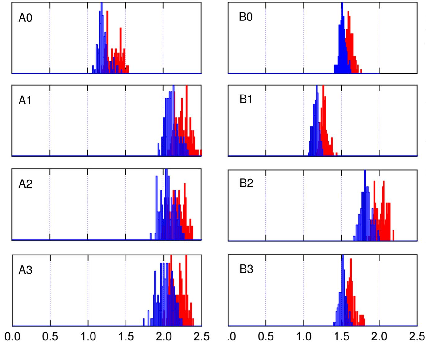
noise consistently higher for channels connected to wirebond pads though longer tracks
