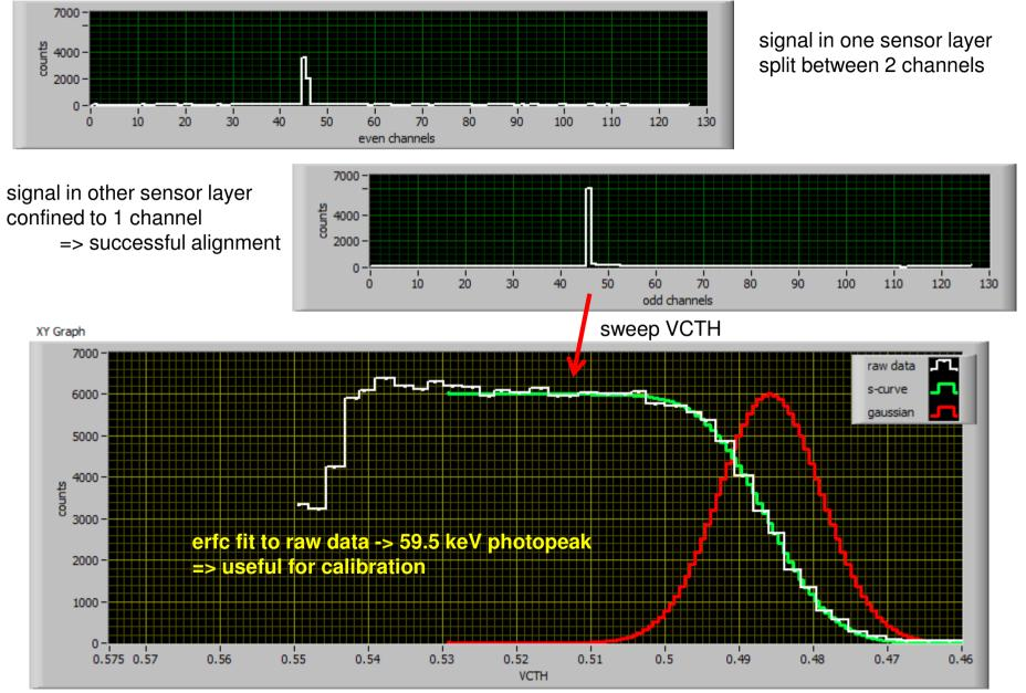
VCTH in Volts (measured using analogue MUX)
