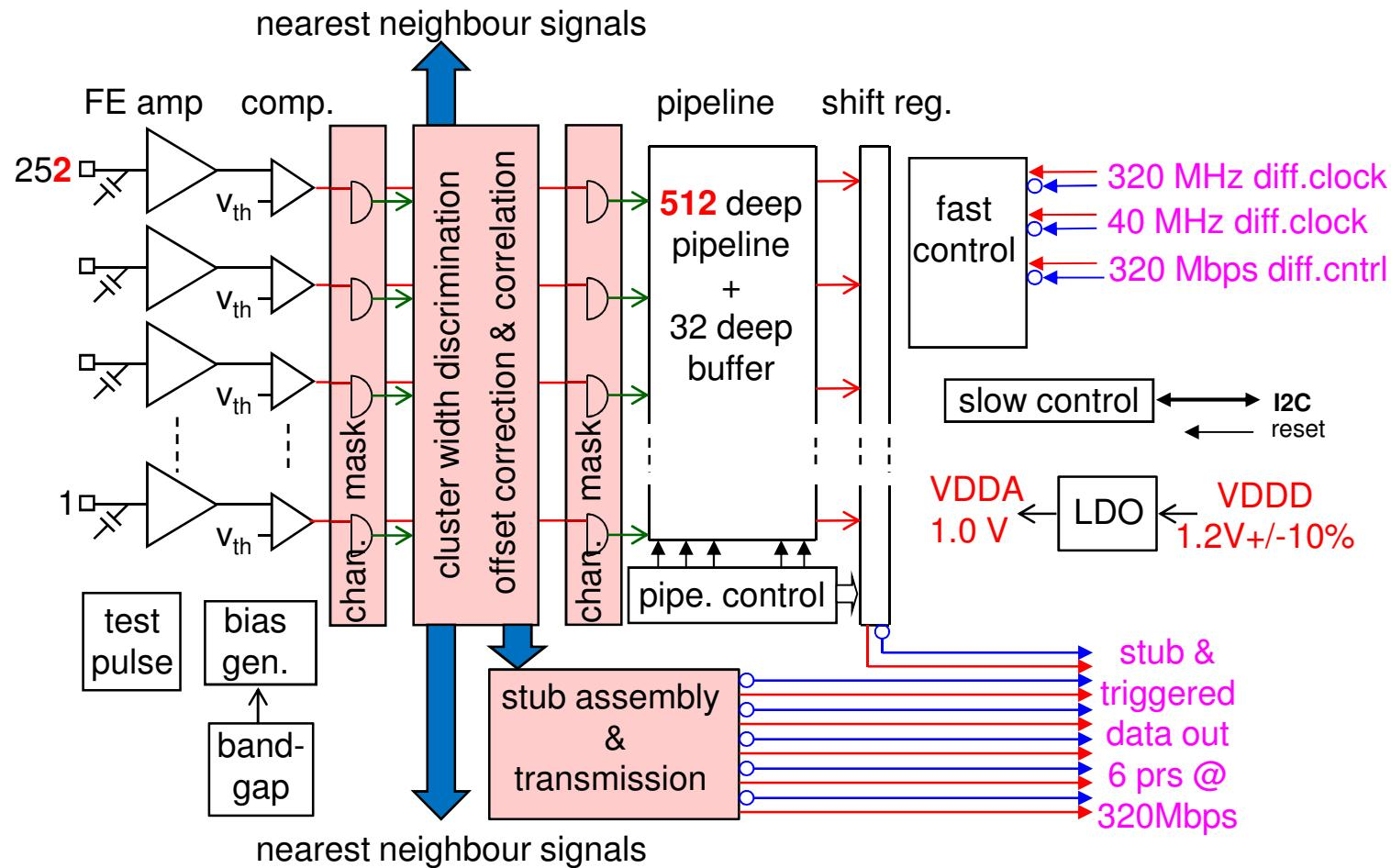
252 channels, 512 deep pipeline (12.8 us), extra chan. mask before pipeline, stub assembly and transmission, all differential I/O, 1 MHz trigger rate capable,
