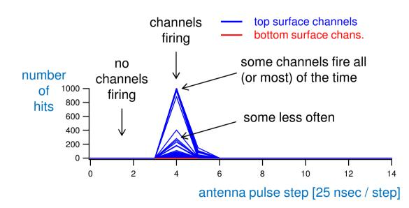
example result for 1V step on top surface antenna
