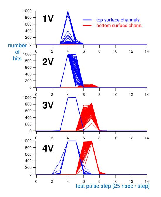
varying antenna signal edge amplitude from 1 to 4 Volts
