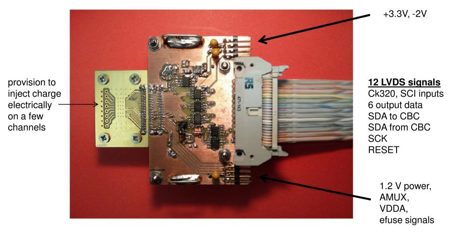
can be connected to VME DAQ and control system
