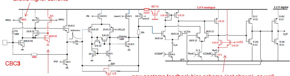
new preamp cascode bias scheme to eliminate "shadow effect"
