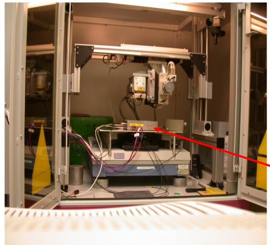
perform more detailed tests (incl. irradiation) on chips already passed wafer test
