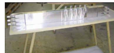
lead layer with light guides
