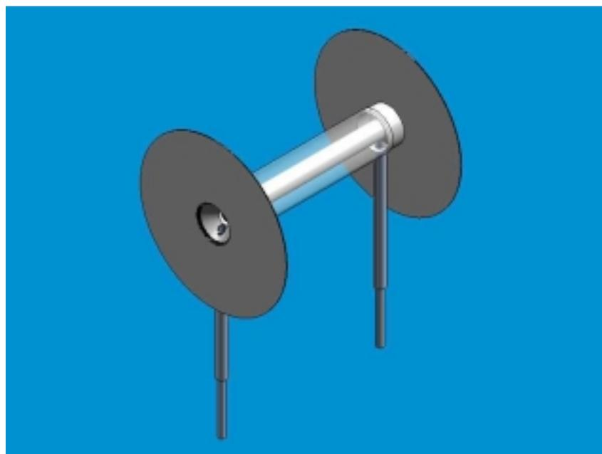
Lens assembly w/ current discs and the primary and secondary coils
