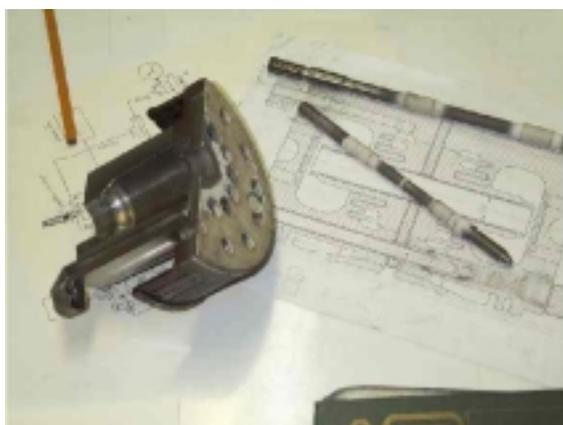
BINP liquid lithium lens, opened lens lithium vessel and the entire system.
