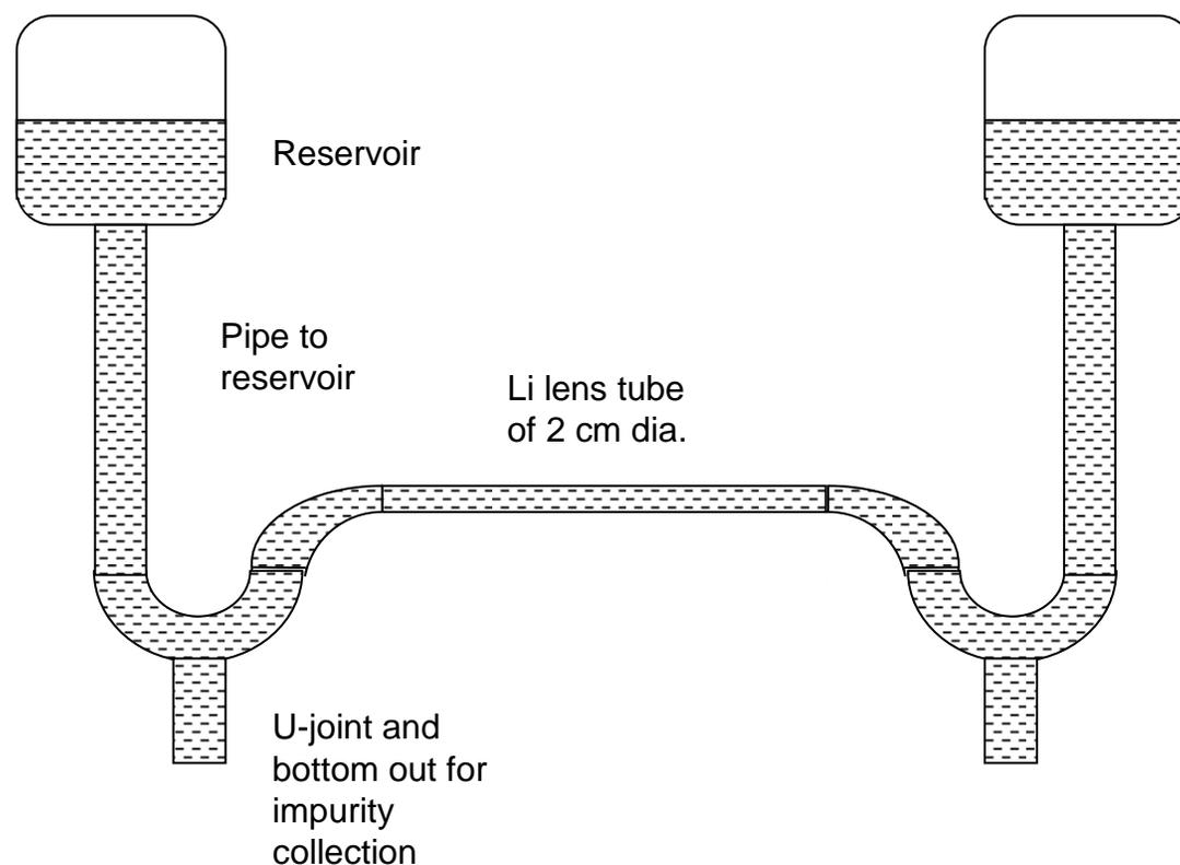
Conceptual Design w/ two reservoirs for push-pull thermal cooling action.
