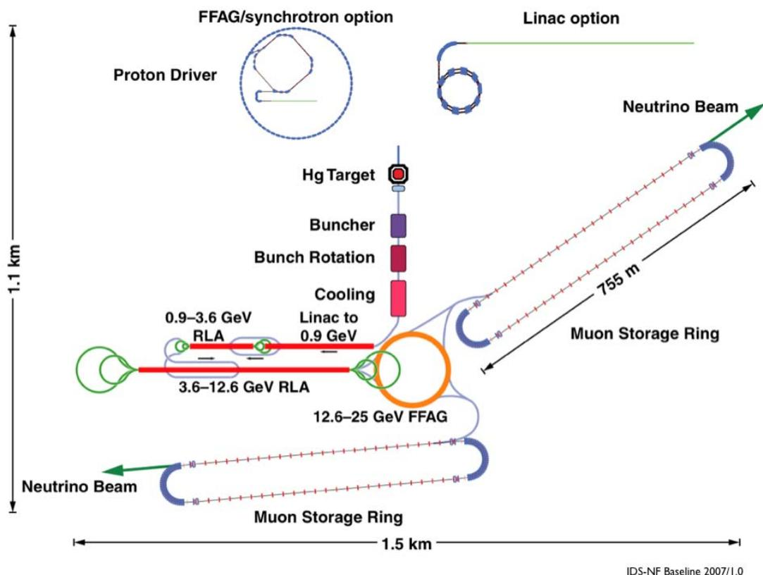
Figure 1: Schematic drawing of the ISS baseline 2007/1.0 for the Neutrino Factory accelerator complex [1]. The various systems have been drawn to scale.
