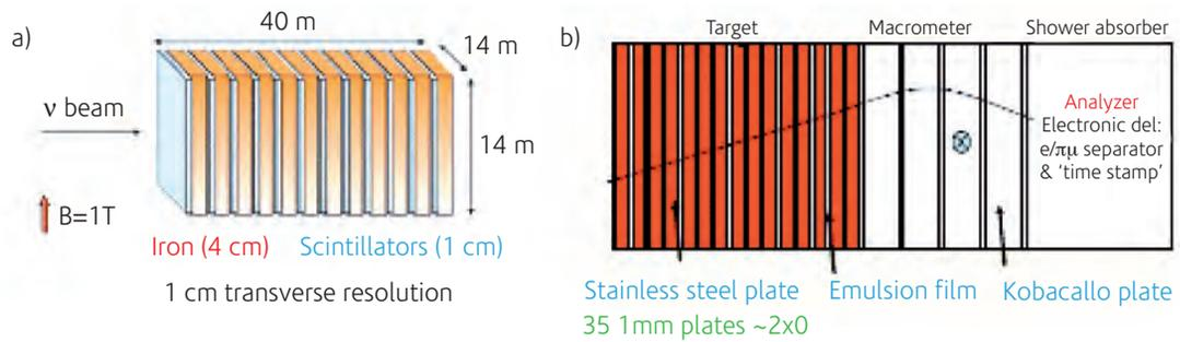
Figure 4: A possible detection system for a high energy neutrino beam from a Neutrino Factory incorporating a MIND (a) followed by a MECC (b) for tau detection<sup>[16]</sup>.
