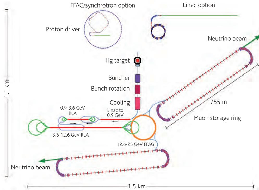
Figure 5: Baseline configuration for the Neutrino Factory resulting from ISS Study<sup>[19]</sup>.
