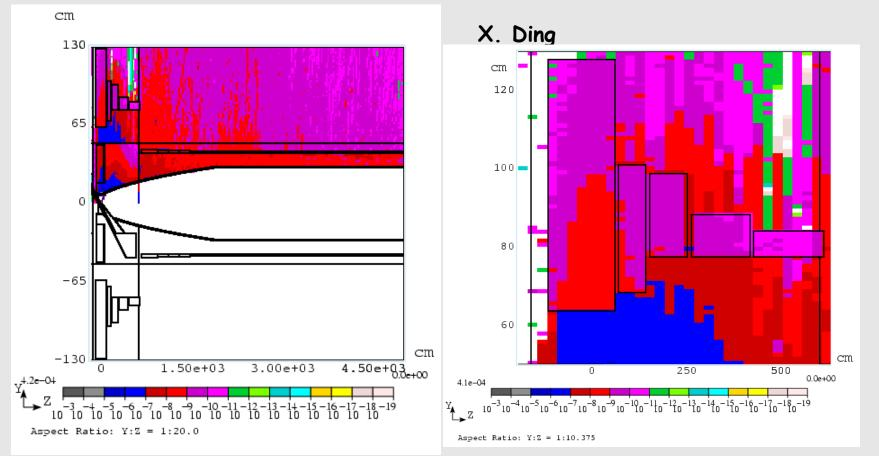
Enhanced shield can decrease the power deposition in SC1 coil from 22.1kW to 4.8kW. By replacing the Res Sol by WC shield, the power deposition in SC1 coil can be decreased further to 1.3kW.
