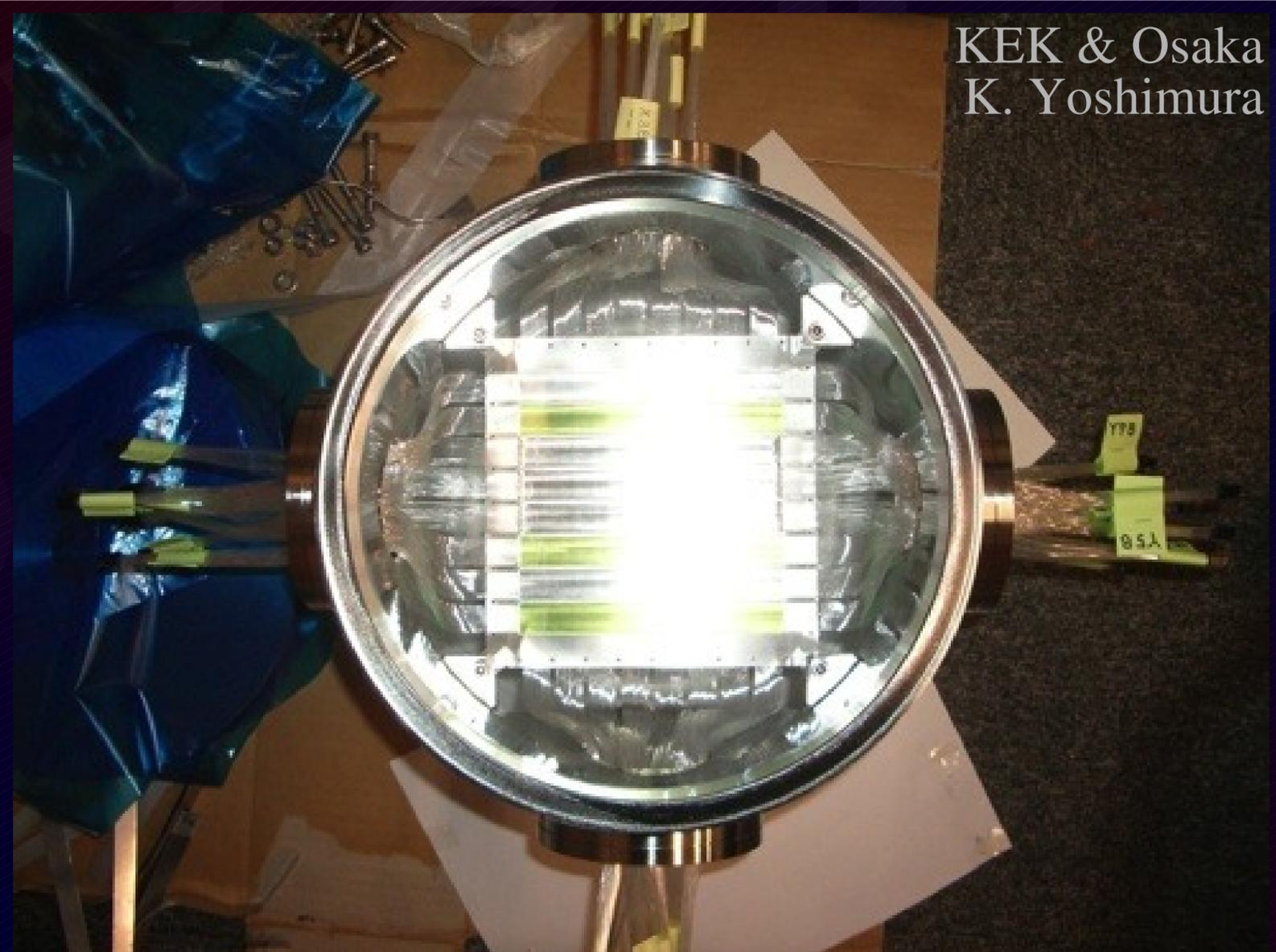
Beam Monitor for Beam Extinction Tests and Measurements at J-PARC
